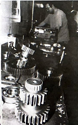
First-year students like Russell Bill (background) in the Diesel Equipment Mechanics program get practical experience in tearing down and rebuilding heavy equipment transmissions in the program's transmission lab.
